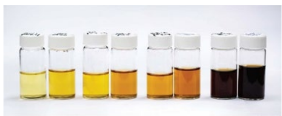
Figure 3: Photos of GQDs from raw and clean coal samples. Image pairs (left to right): lignite, subbituminous, bituminous, and anthracite. In each pair, the left sample is from raw coal and the right sample is from clean coal.
