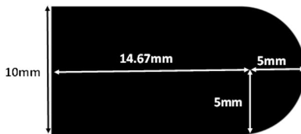
Figure 2: A simple design for a mold to create a silver pattern. The mold was composed of a rectangular pattern size of 10 mm  $\times$  14.67 mm with a semi-circular pattern with radius of 5 mm.
