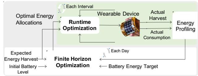
Figure 1: Overview of the energy allocation algorithm
