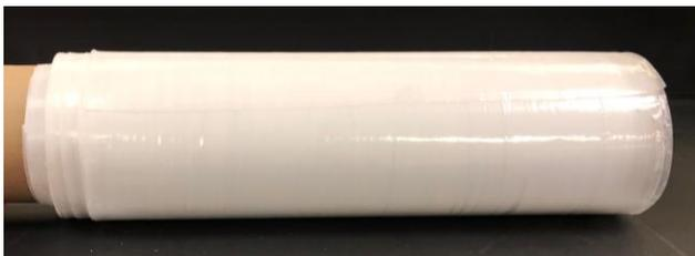
Figure 1. Flexible film consisting of 65 alternating layers of PA6 and TFP glass.
