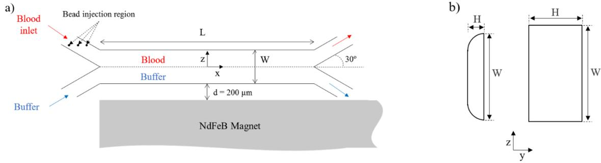
**Figure 1.** a) Schematic view the continuous-flow magnetophoretic separator; b) Generic cross-section of the microchannels.
