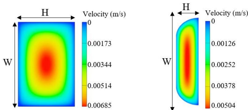
**Figure 2.** Velocity distribution in a section perpendicular to flow direction for rectangular (left) and U-shaped (right) channels.
