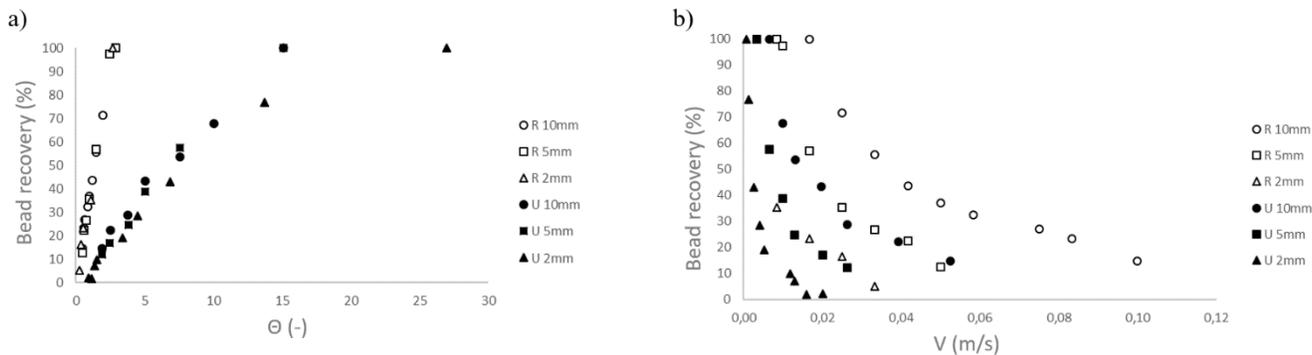
**Figure 3.** a) Influence of cross-sectional areas in bead recovery and b) Influence of fluid velocity in the system performance for rectangular (R) and U-shaped (U) channels.
