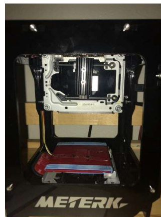
Figure 3: Fabrication of Graphene Electrodes Using Laser Engraving
