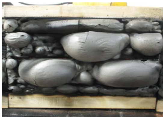
Figure 3: Armstrong’s Class A Coating After Successful E84 Steiner Tunnel Test
