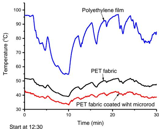
Figure 5: Results of the outdoor solar heat shielding test.
