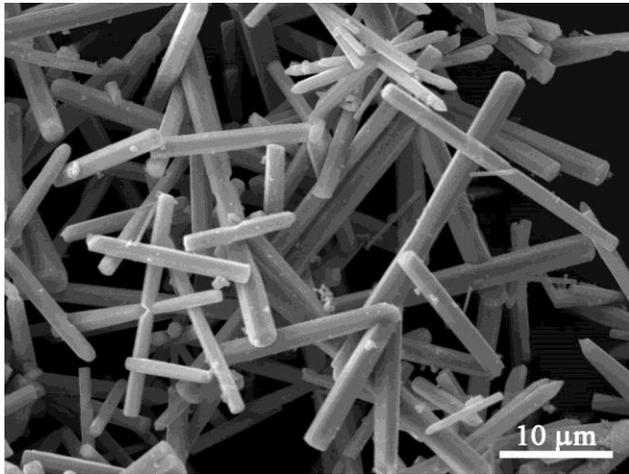
Figure 2: SEM image of Al-ZnO microrods.
