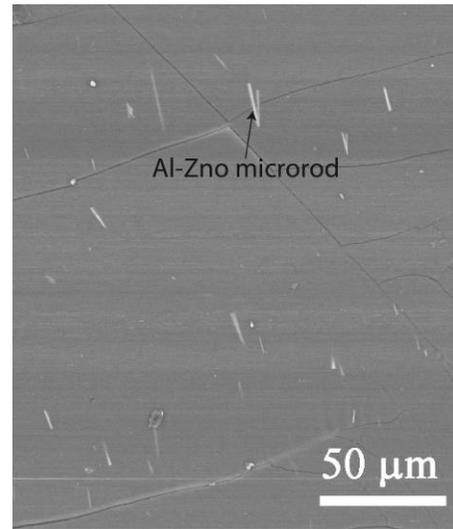
Figure 3: SEM image of the parallel alignment of Al-ZnO microrods coating on the PET fabric.
