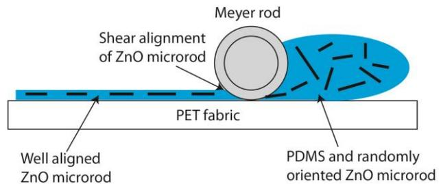
Figure 4: the alignment mechanism of microrods
