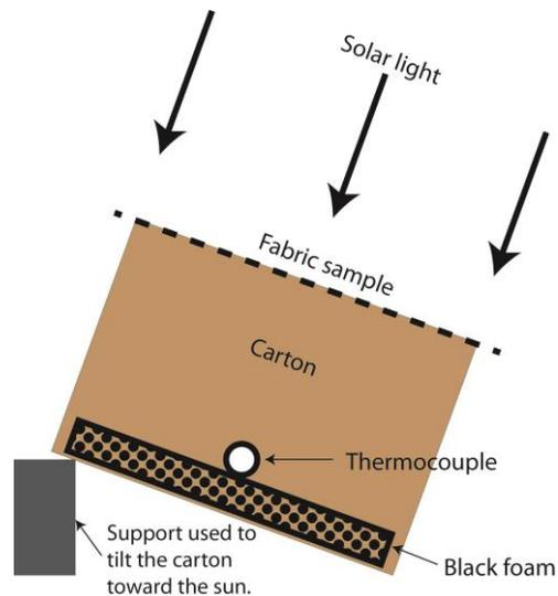
Figure 1: Scheme diagram of the experimental setup for outdoor solar heat shielding test.
