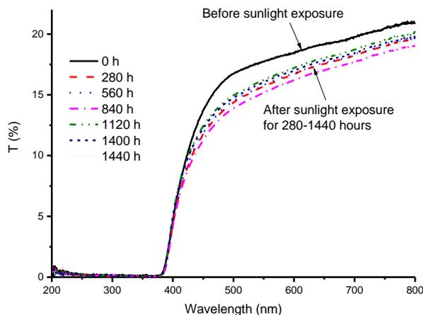
Figure 6: The UV/Vis spectra of the PET fabric coated with the microrods after sunlight weathering test.
