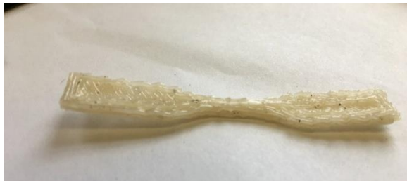
Figure 3: Dog bone printed at a bed temperature of 100 °C
