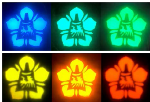
Figure 4: The driving of DHFLC: a) the top three waveforms are the applied signal to the sequential RGB LED, and the bottom waveform is the combined appearance of the DHFLC cell with compound 3. b) Top: target colorful image, middle: deformed-helix ferroelectric liquid crystal cell, bottom: one frame consists of three R-G-B sub-images. c) Photographs of the developed Field-Sequential Color Liquid Crystal Display operated at a color frequency of 500 Hz (i.e., a frame frequency of 166 Hz) of SmC* 3. The device size is 2 cm \times 4 cm, and the effective electrode area is 1 cm \times 1 cm.
