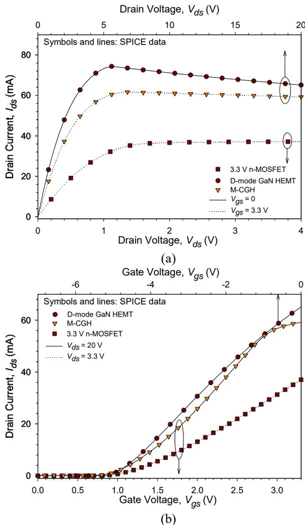
Figure 3: Comparison of (triangle) M-CGH with (circle) D-mode GaN HEMT and (square) n-MOSFET in the simulated (a) transfer and (b) output characteristics.
