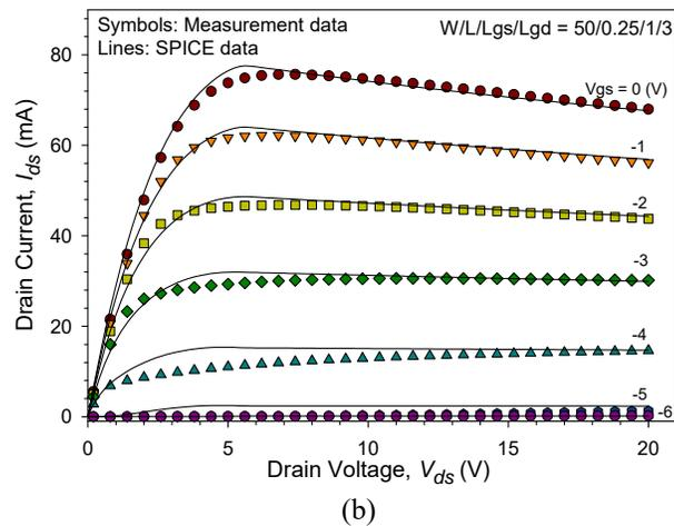
Figure 1: Comparison of the (lines) SPICE data with (symbols) measurement data in the (a) transfer and (b) output characteristics of a 2-finger DGaNH.
