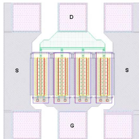
Figure 4: One of the demonstration structures to show a 4-finger M-CGH configuration with D, S, and G terminals in PCELL formation.
