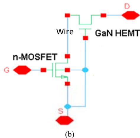
Figure 2: The design of M-CGH with a 2-finger DGaNH in series connection with a 2-finger n-MOSFET. It shows the symmetric design in (a) layout with metal connections and (b) schematic with wire connections between DGaNH and n-MOSFET terminals.
