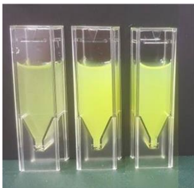
Figure 4: Curcuminoids oil nanoemulsions: (a) coarse emulsion, (b) microfluidization nanoemulsion, and (c) ultrasonication nanoemulsion.
