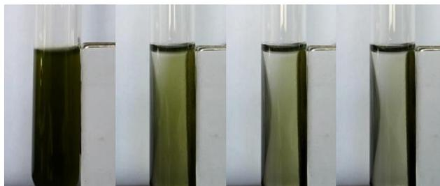
Figure 2 Photographs for the time-lapse magnetic separation process of *C. pyrenoidosa* using CPAM-Fe<sub>3</sub>O<sub>4</sub> particles. From left to right: 0 s; 30 s; 60 s; 120 s.
