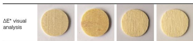
Figure 1: Visual analysis of samples colour variation. From left to right samples UncoatAD, 2hCoat100, 1hCoat100 and CoatAD are showed.
