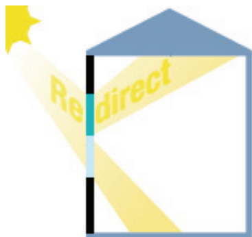
Figure 8: Illustration showing Solar Energy redirected further into building with micro-structures on window.
