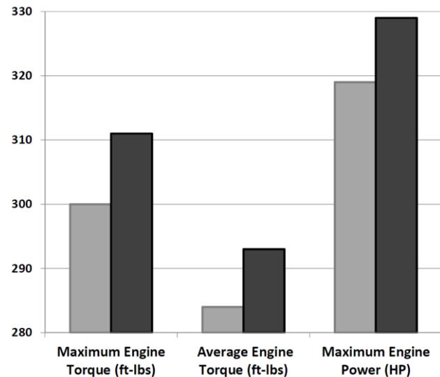
**Figure 4.** Dynamometer tested improvements in vehicle performance metrics, measured as torque and horsepower. Gray bars represent vehicle performance prior to treatment with TriboTEX Engine Coating. Black bars represent measured performance 500 miles after TriboTEX Engine Coating treatment. **Test Vehicle:** 2015 Ford Mustang
