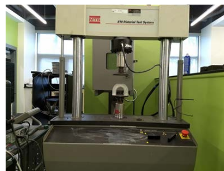
Fig. 4 Unconfined compression test using the MTS loading machine.
