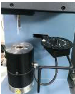
Figure 1. Sample of polyurethane control located on TGA instrument
