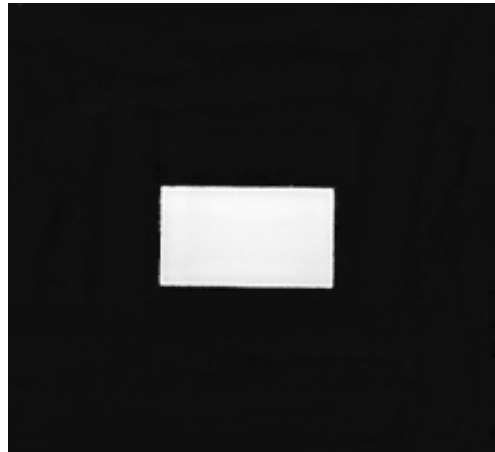
Figure 4: Example of a rectangular pattern printed with high refractive index scatterer-containing formulation.
