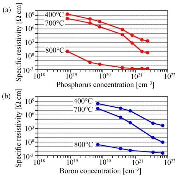
Figure 5: Specific resistivity of the doped silicon films with different annealing temperature and dopant concentration. (a) n-type silicon and (b) p-type silicon.
