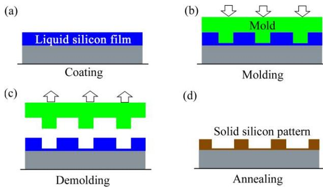
Figure 2: Imprint procedure of liquid silicon. (a) Liquid silicon was spin-coated on a substrate and cured at 160°C for 5 min. (b) A mold was pressed into the film at 10 MPa and at 160°C for 10 min, followed by the temperature was raised up to 200°C and kept it for 10 min with maintaining the pressure at 10 MPa. (c) The mold was released after cooling down below 160°C. (d) The resultant film was annealed at 400–800°C for 10 min to complete the liquid-to-solid conversion.
