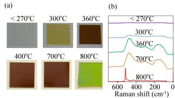
Figure 3: Solidification of liquid silicon film on a flat substrate. (a) Photographic image of solution-processed liquid silicon films with a thickness of 80 nm. The annealing temperature was from 270 to 800°C. (b) Raman spectra of the films. The spectra for the films with 400–700°C show amorphous silicon, whereas that for the film with 800°C shows polycrystalline silicon.
