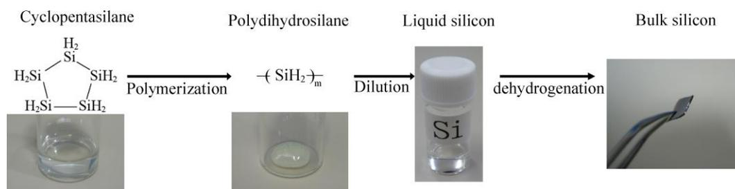
Figure 1: Preparation route for liquid silicon and solution-processed silicon.
