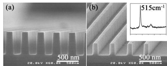
Figure 6: SEM images of (a) mold and (b) imprinted silicon lines after annealing at 800°C. Raman spectrum of the patterns are inserted in upper right.
