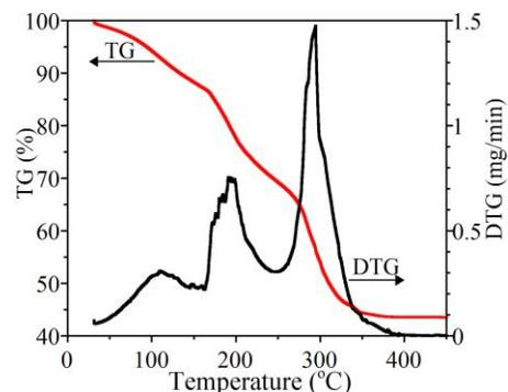
Figure 4: TG and DTG signals of polydihydrosilane as a function of heating temperature. Reproduced with permission from ref [13]. Copyright 2012 Elsevier B.V.
