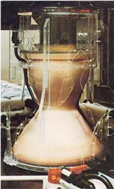
Figure 3 Combustion chamber undergoing electroplating. (Image: Google Images)
