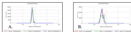
Fig. 1. A). Zeta Potential Analysis for GNRs. Average ZP value= -20.7667 mV. B). Zeta Potential Analysis for FITC-Conjugated GNRs. Average ZP=-34.7333 mV.
