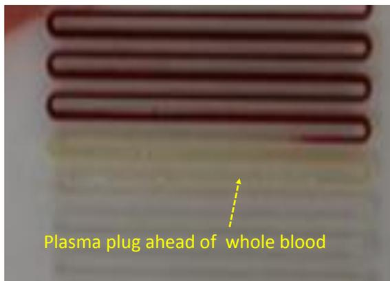
Fig.5. Details of the plasma plug in the open rectangular channel. The volume of plasma is approximately 15  $\mu$ l.
