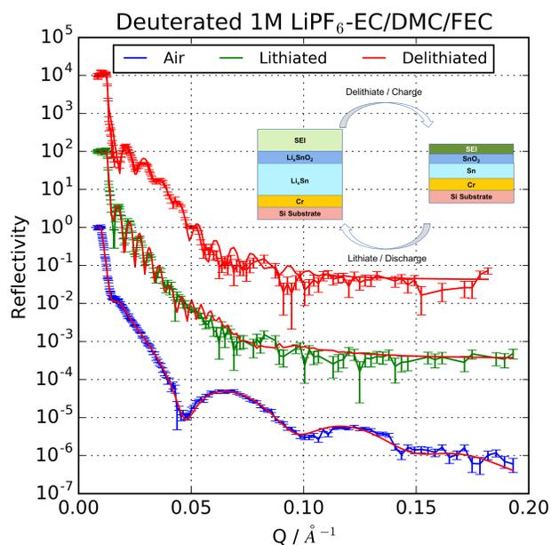
Figure 2: Neutron reflectometry data and respective model fits on tin anode samples and schematic of the changing thickness/SLD of the SEI between the lithiated and delithiated states (inset figure).
