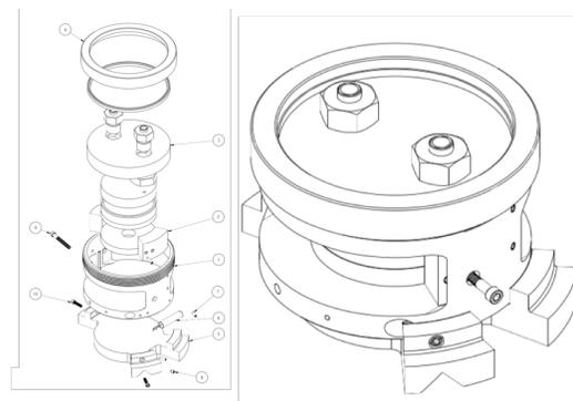
Figure 1: Schematic of electrochemical reflectometry cell.
