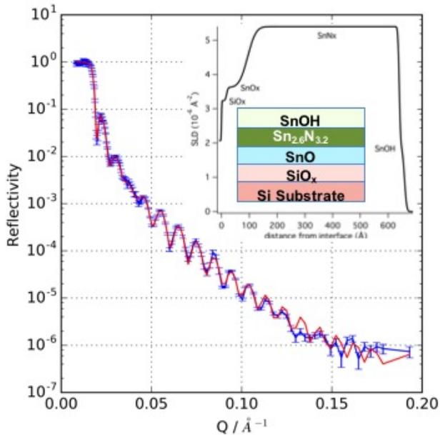
Figure 3: Neutron reflectometry and model fit of tin nitride thin film. Inset scattering length density profile and schematic of thin film structure.
