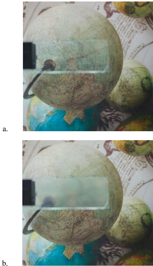
Figure 1. a passive DHR (Dynamic Heat Reduction) prototype device. (a) "Off" state, (b) "On" state
