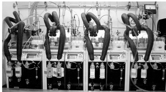
Figure 1: Custom automated reactor system for combinatorial approaches to functional photonic nanomaterials discovery and optimization located in the Center for Integrated Nanotechnologies (CINT) Gateway Facility, Los Alamos National Laboratory.
