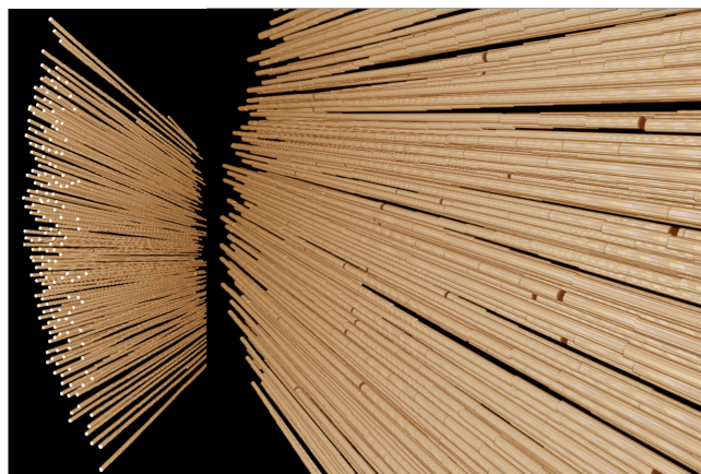
Figure 3: 3D rendering of solid fibers detected from a composite sample, along with detected fiber failures (gaps).
