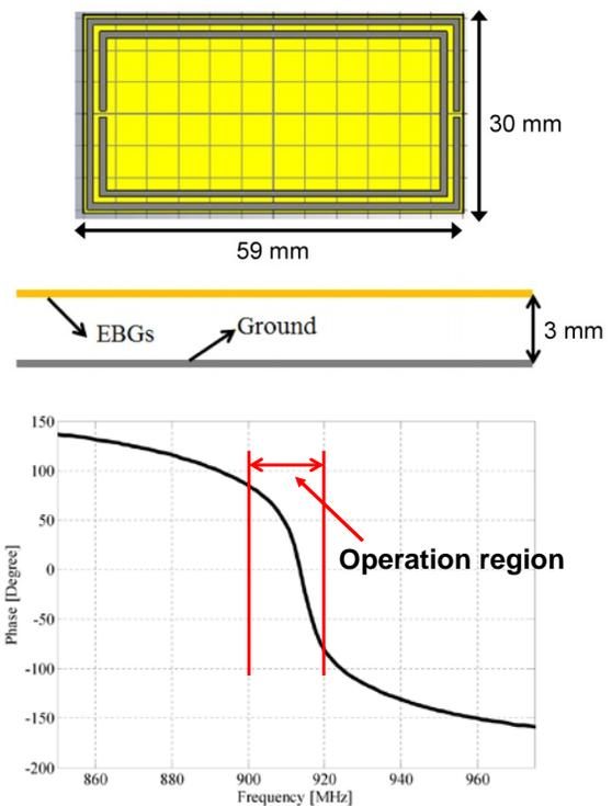
Figure 7. EBG unit cell (top) and the resulting simulated reflection phase (bottom).
