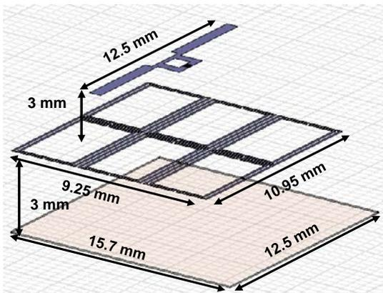
Figure 8. Dipole antenna matched to the RFID chip on top of the designed SRR-based EBG surface.
