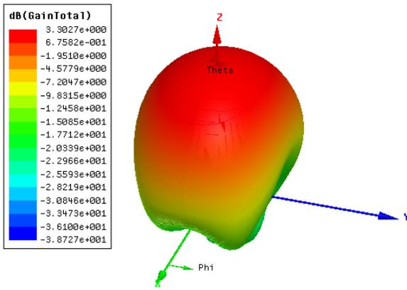
Figure 6. Radiation pattern of CNT-loaded patch antenna in CST simulation software.
