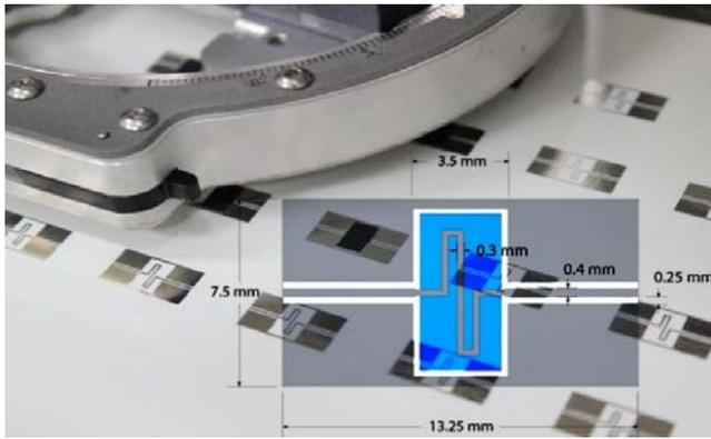
Figure 10. Inkjet printed magnetic nanomaterial on meandered inductor on photopaper.
