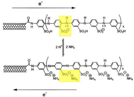
Figure 3. Mechanism of interaction of PABS-SWNT with  $\text{NH}_3$ . The arrows indicate charge transfer between SWNT and PABS. [3]
