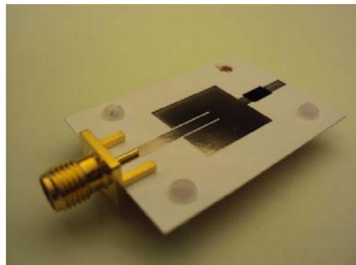
Figure 5. Fabricated prototype of inkjet-printed CNT and patch antenna on photopaper.
