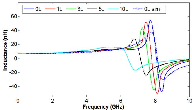
Figure 11. Measured inductance for varying number of layers of nanomaterial, showing shift in SRF.
