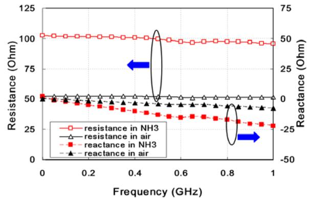
Figure 4. High frequency impedance characterization of CNT in air and in ammonia gas.
