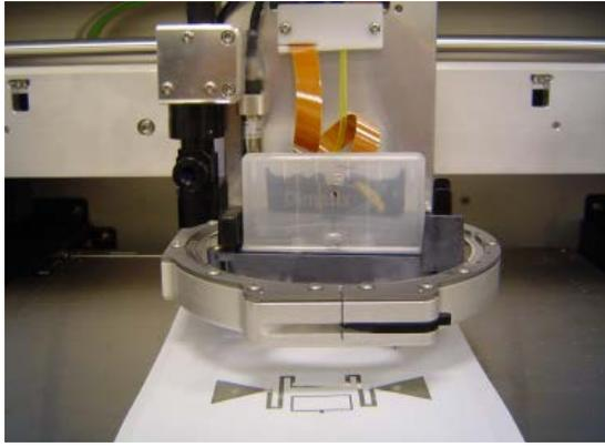
Figure 1. Fujifilm Dimatix materials printer printing conductive ink on paper substrate.
