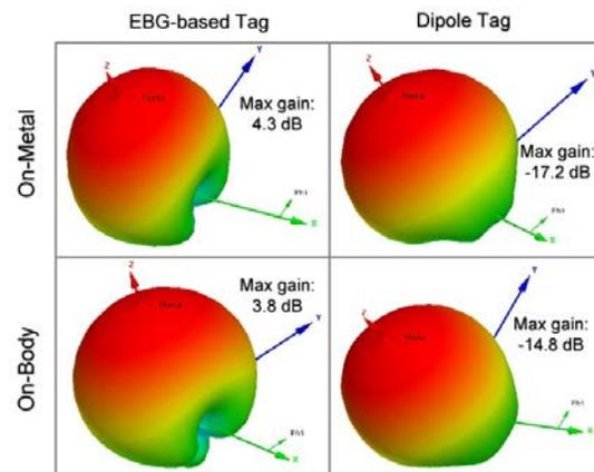
Figure 9. Simulated 3D radiation patterns of the EBG-backed and dipole Tags on both metal and body.
