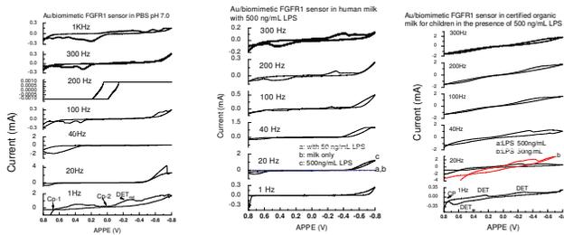
Fig 3 (L) Illustrates the frequency affects from 1 Hz to 1 KHz on hysteresis of the i-V curve of the memristor in PBS. Fig. 4 (m) depicts frequency affects with 500ng/mL LPS in human milk against control. Fig. 5(R) depicts the i-V curve in the presence of 500 ng/mL LPS in organic milk.
