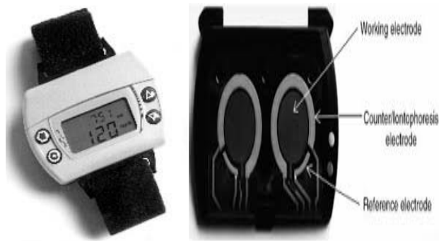
Figure 2. A GlucoWatch G2 Biographer designed by Cygnus Inc.
