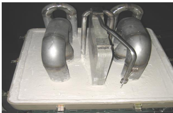
Figure 2: Plasma reformer for 10 kW SOFC
