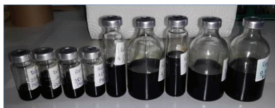
Picture 4: Synthesized PbS QDs with different control parameters via continuous flow reactor.
