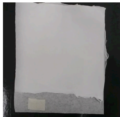
Figure 3 : Photograph of nonwove nanofiber based on recycled PET.
