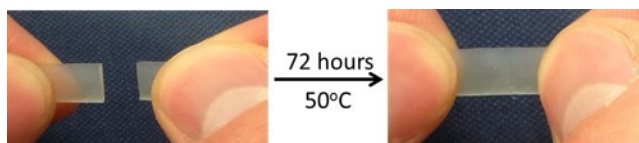
Figure 6. Functionalised h-TPE demonstrating self-healing properties. The sample was bisected, rejoined, and then held at 50°C for 72 hours.
