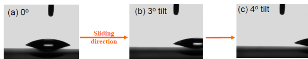
Figure 3. Snapshots of a sliding hexadecane droplet (~10 \mu L) on a polyurethane coating containing 7.5% of SilClean3700.
