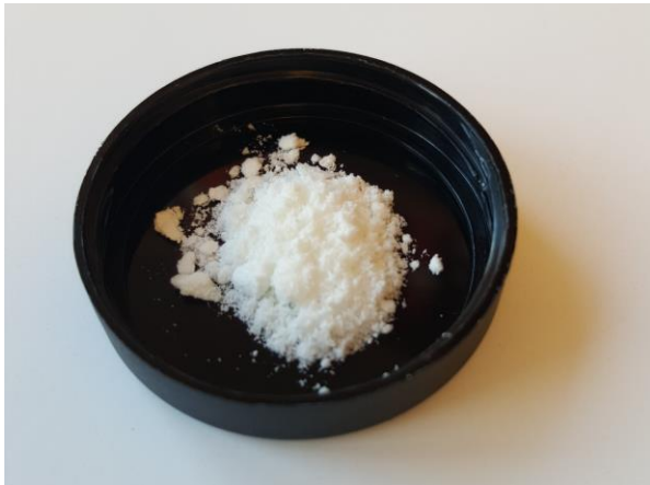
Figure 4: Dried oil filled powder for mixing with water or to be used as is to deliver encapsulated material to skin.
