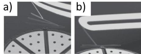
Figure 7: SEM images showing the spring deformation (a) prior to actuation and (b) during actuation of the bimorph.
