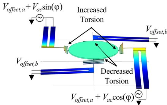
Figure 5: FEM simulations of the mirror showing the difference in mechanical strain in the serpentine springs connected to bimorph legs with a nonzero offset power  $V_{offset,b}$  with an overlay of the differential driving circuit.
