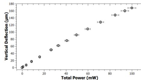
Figure 4: The vertical deflection of the micromirror is shown as a function of total power dissipated.
