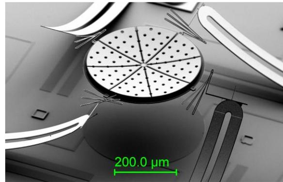
Figure 1: SEM image of large range tip-tilt-piston micromirror with integrated variable focus.
