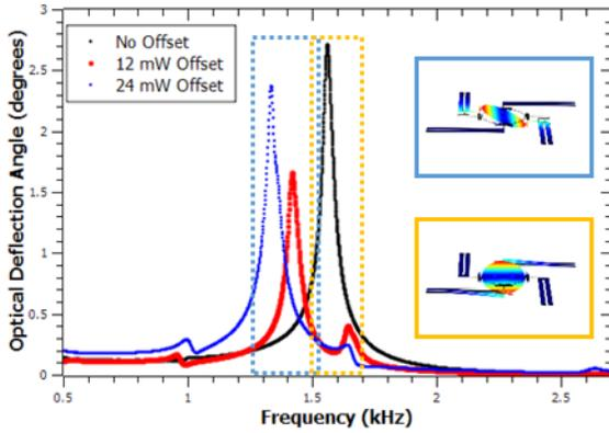
Figure 9: Measured frequency response data for varying  $V_{offset,b}$  for a power of 0 mW, 12 mW and 24 mW in each of the offset bimorphs. Insets are simulated mode shapes.
