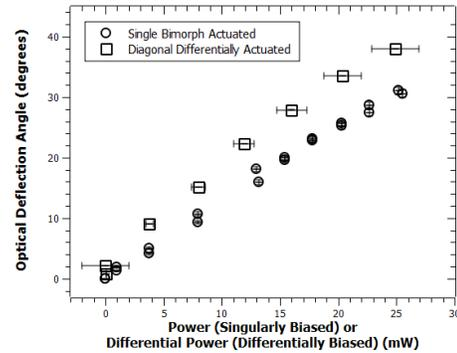
Figure 3: The optical deflection for diagonal differential actuation (square), singular actuation (circle). Some error bars are too small to be seen.
