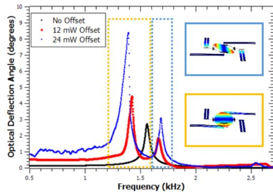
Figure 8: Measured frequency response data for varying  $V_{offset,a}$  for a power of 0 mW, 12 mW and 24 mW in each of the offset bimorphs. Insets are mode shapes simulated in COMSOL.
