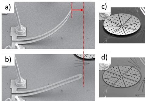
Figure 2: SEM images showing a bimorph leg (a) unactuated and (b) actuated and the variable focus mirror (c) unactuated and (d) actuated.
