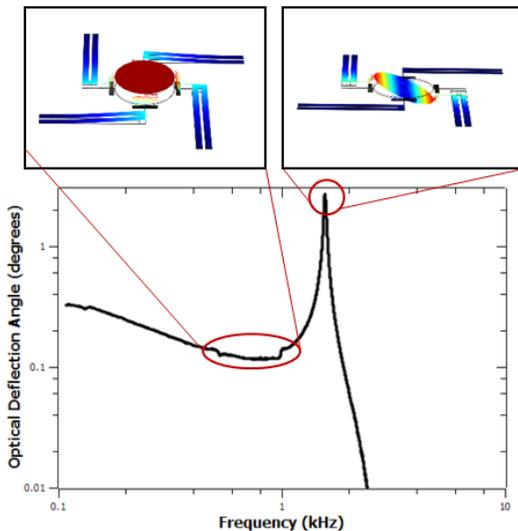
Figure 6: The measured frequency response data with zero offset voltages is provided showing the corresponding mode shapes as simulated in COMSOL.
