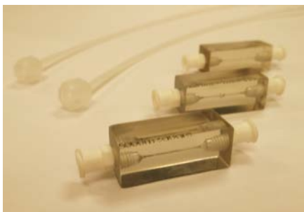
Figure 5: 3D printed chips with shaped internal cavities
