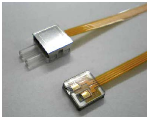
Figure 3: The 7 x 7 mm micro pumps
