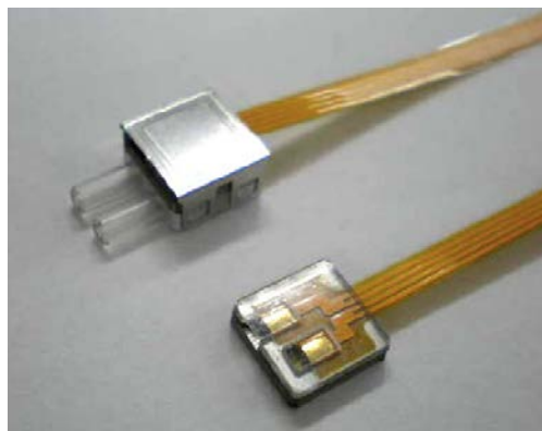
Figure 3: The 7 x 7 mm micro pumps
