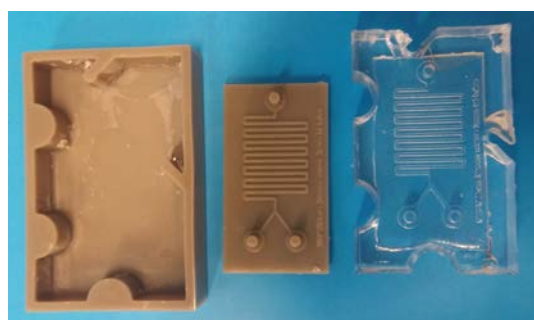
Figure 8: (left) a mould housing was used to position the pattern, (middle) the pattern for the moulding and (right) the final PDMS cast flow-chip prior to trimming
