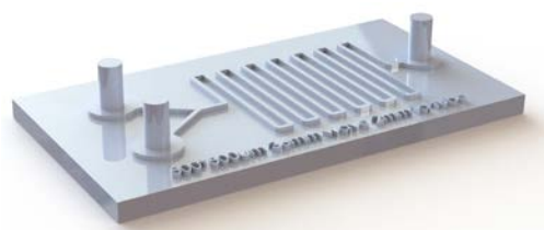
Figure 7: 3D CAD of a printed mould
