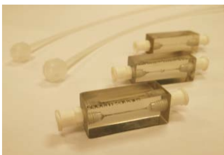
Figure 5: 3D printed chips with shaped internal cavities
