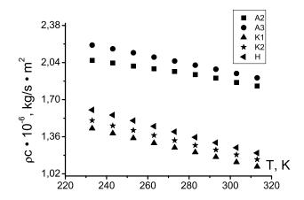
Figure 1: Acoustic impedance of different magnetic nanofluids *versus* temperature.
