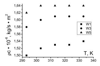
Figure 2: Acoustic impedance of water-based versus temperature.
