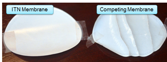
Figure 7—ITN’s membrane remains intact after drying, while competing membranes crack and wrinkle when dried.
