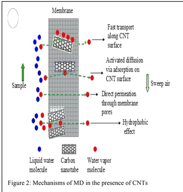
Figure 2: Mechanisms of MD in the presence of CNTs
