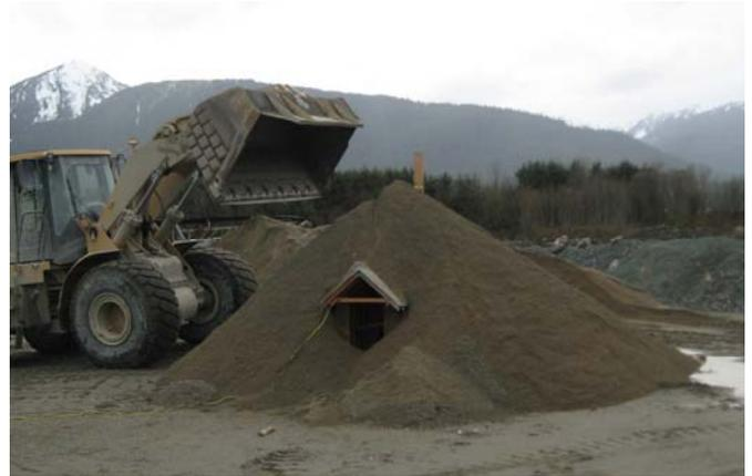
Figure 9. Strength test: 1 m sand on top. No visible damage. Dial indicators inside the uninsulated concrete shell showed ~ 0.010” deflection at horizontal diameter and vertical apex.
