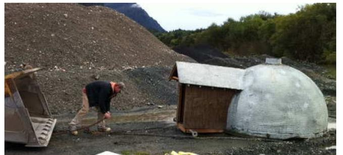
Figure 10. Seismic test: repeated ~2.7 g shocks. Wire rope wrapped around foundation ring. No visible damage.
