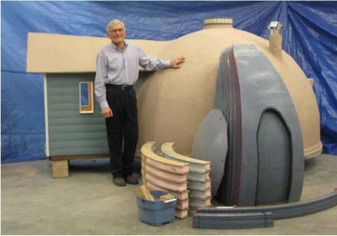
Figure 1. Complete forms set, for foundation ring and dome. First prototype: proof-of concept one-third scale model, with skylight, window, chimney
