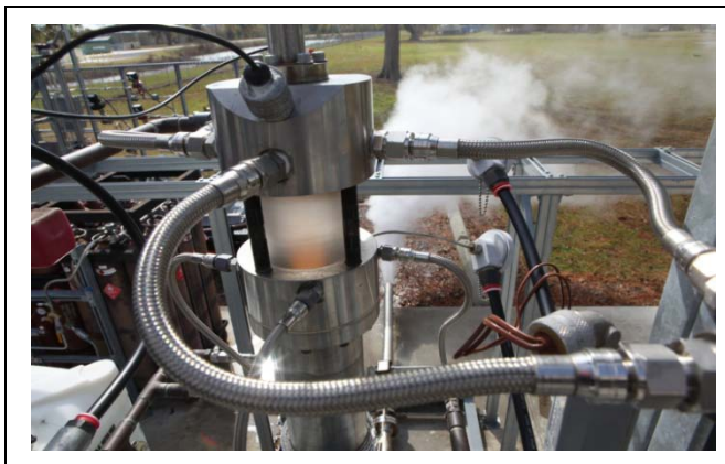
Figure 2: 1-MMBtu/h -100 psi steam generator in operation at HydroFlame facility in Baton Rouge
