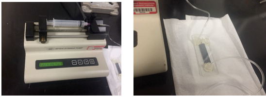
Figure 8: Fluid flow test setup
