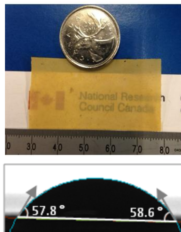
Figure 4: A BNNT-buckypaper-epoxy composite ( > 30 wt.% BNNTs, \sim 60 \mu\text{m} thick) and contact angle image showing the initial contact angle for the epoxy with BNNT buckypaper at room temperature. Adapted from [7] with permission.
