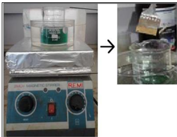
Figure 2: Electroless plating experimental setup
