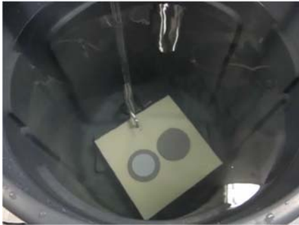
Figure 4: Immersion of treated and untreated samples at depth of 1 meter under water.
