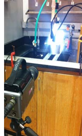
Figure 2: High speed camera with backlight used to image droplets.
