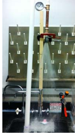
Figure 1: Rain test of a thermoset rubber using BETE nozzle.
