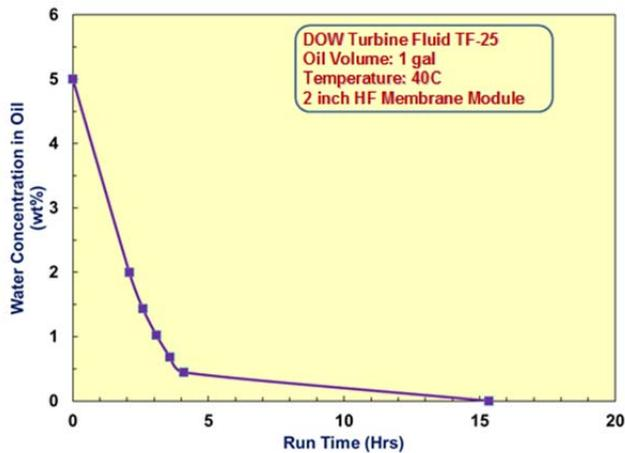
Figure 4. EAL drying with membrane dehydrator
