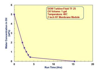
Figure 4. EAL drying with membrane dehydrator
