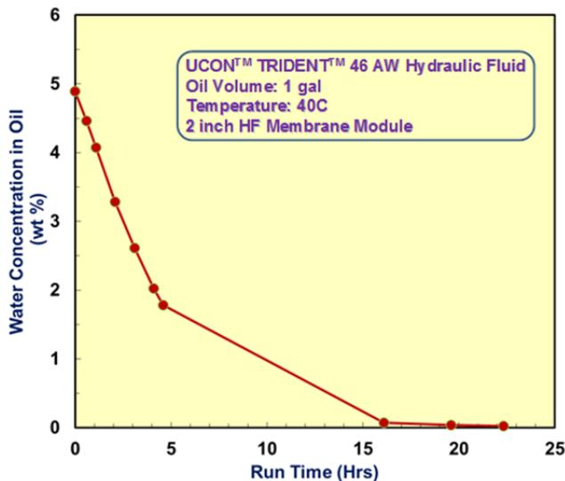
Figure 5. Test run with EAL hydraulic fluid
