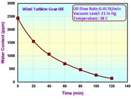
Figure 3. Drying wind turbine gear oil
