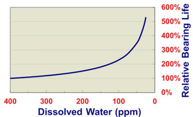
Figure 1. Bearing life vs. Dissolved water concentration
