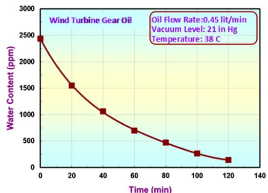
Figure 3. Drying wind turbine gear oil
