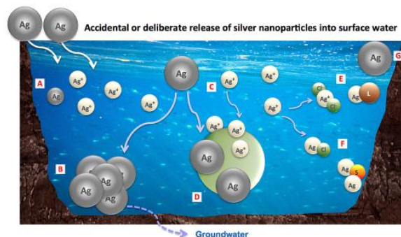
Figure 1 Possible fates of silver nanoparticles in surface waters: (A) Dissolution process leading to free ions release and smaller particles; (B) Aggregation into larger particles, which may settle out of the water, depending on the aggregate size; (C, D) Adsorption of released Ag^+ and nAg , respectively, onto other solids present in the water; (E) Formation of soluble complexes; (F) Reaction with other components in the water, which may result in precipitation; (G) nAg remaining stable.
